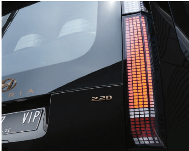
Parametric Pixel Light (LED Rear Combination Lamps)
